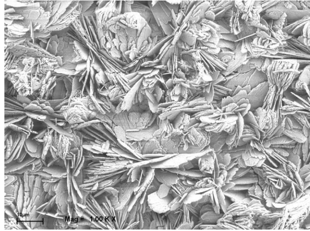
FIGURE 1. SEM of an used Bonit-coated surface.
